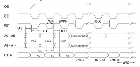
Notes: 1. A6 through A14 must specify the same page address during each high to low transition of WE (or CE) after the software code has been entered.
