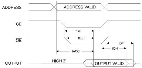
Notes: 1.  $\overline{\text{CE}}$  may be delayed up to  $t_{\text{ACC}}$  -  $t_{\text{CE}}$  after the address transition without impact on  $t_{\text{ACC}}$ .
