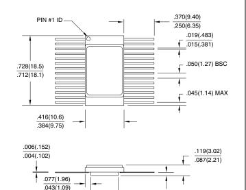
**32J**, 32-lead, Plastic J-leaded Chip Carrier (PLCC) Dimensions in Inches and (Millimeters) JEDEC STANDARD MS-016 AE
