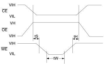
$t_S = t_H = 5 \mu sec (min.)$   $t_W = 10 msec (min.)$  $V_H = 12.0V \pm 0.5V$
